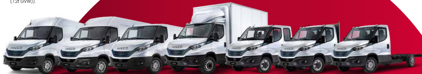
1. Multiple variants of the Iveco Daily to be electrified (Cab, Van, Crew Cab (4.25t-7.2t Gross Vehicle Weight (GVW)), Chassis Cowl and Minivan (7.2t GVW)).
